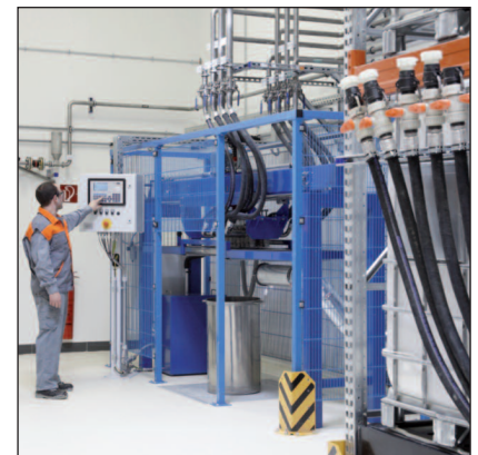
Kleinkomponenten-Dosieranlage Small component dosing equipment
