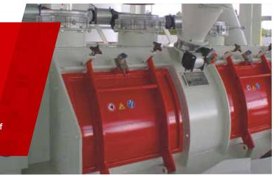
The ploughshare-type mixer is designed for dry mortar materials and "made in Germany". It is available with a useful volume ranging from 101 up to 4,000 l.
